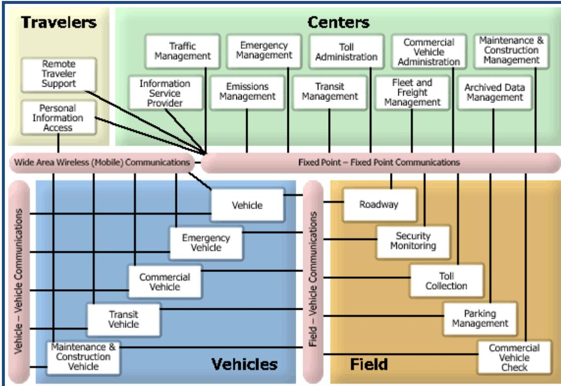
Figure 4-2: High-Level Physical National ITS Architecture
