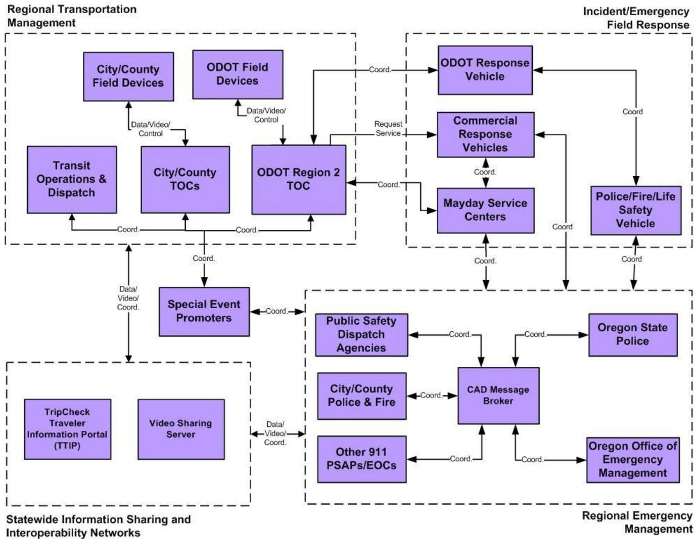
Figure 5-4: Incident & Emergency Management Operational Concept
