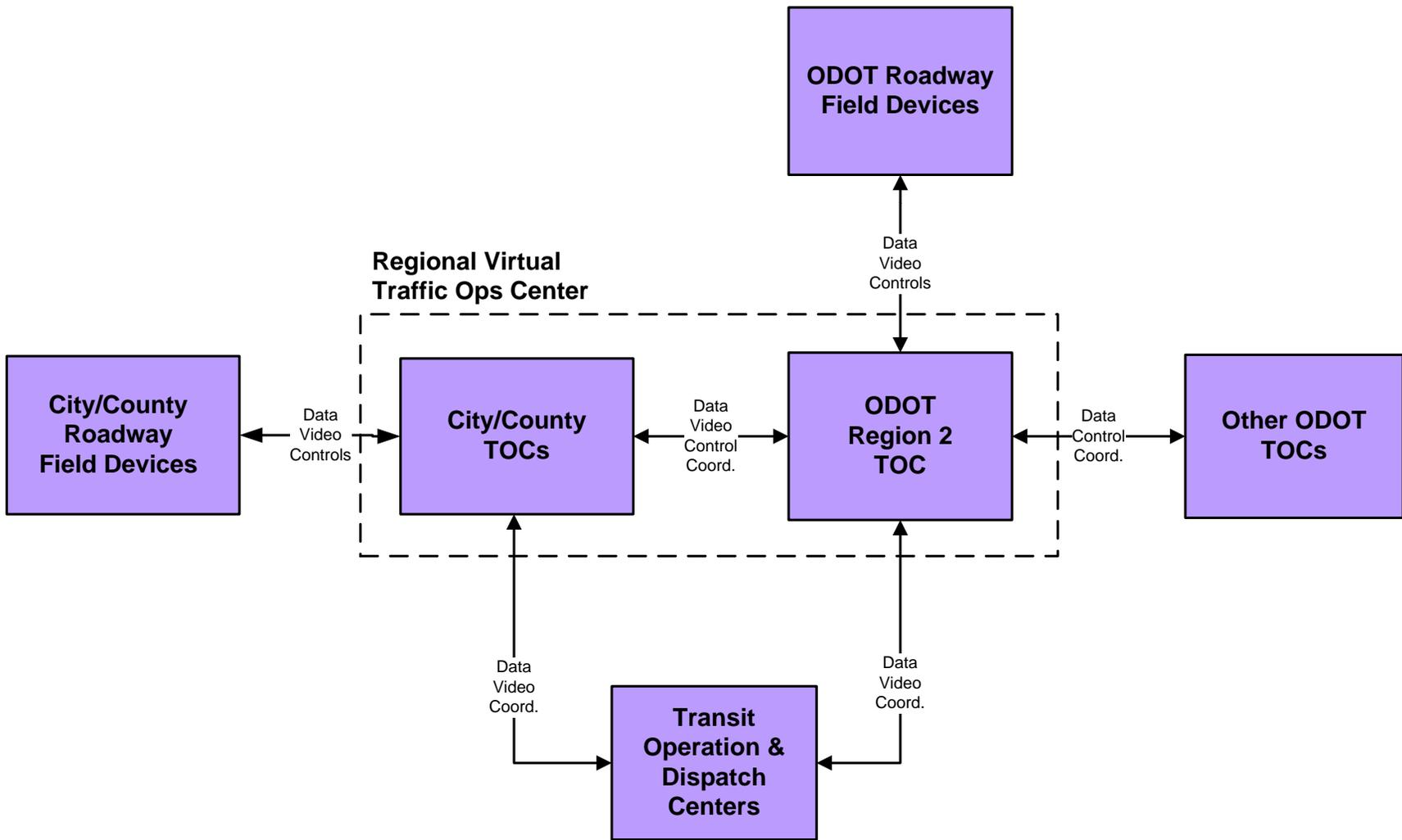
Figure 5-1: Traffic Management & Operations Operational Concept
