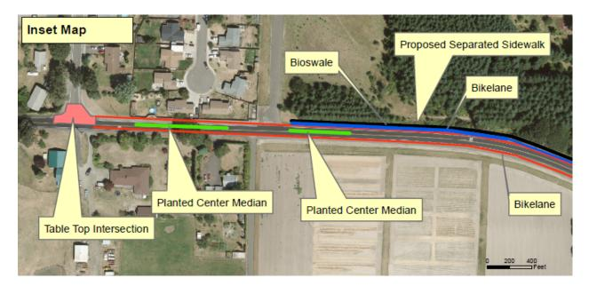
Figure 4: Bicycle and Pedestrian Improvement Plan Conceptual Design
