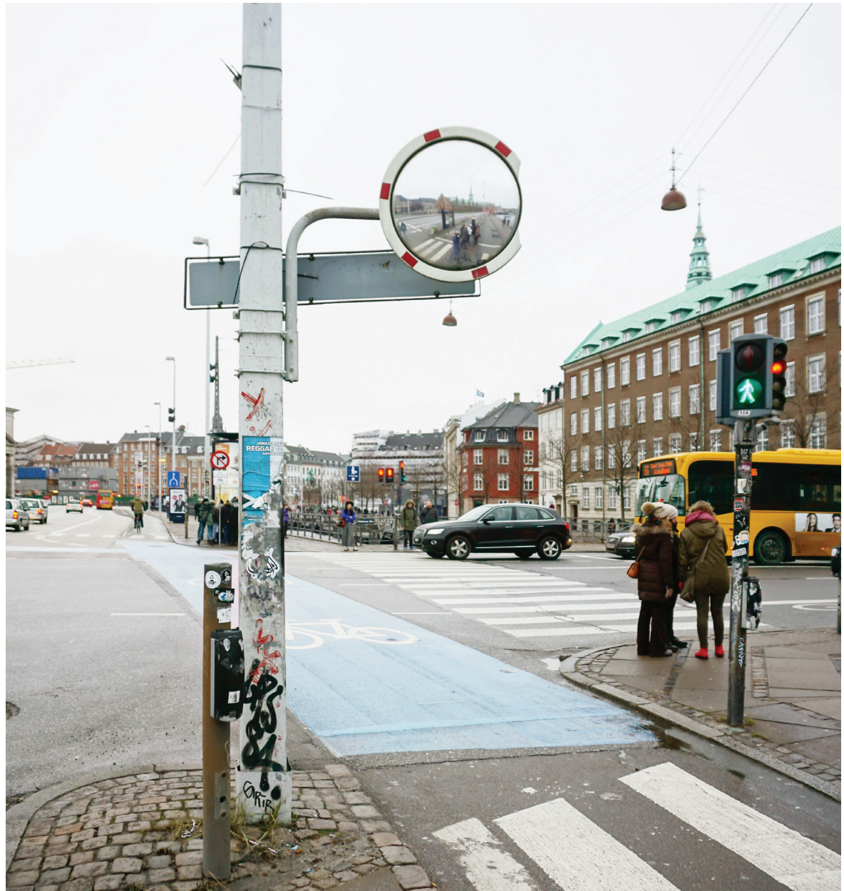
Convex safety mirror mounted to lightpost
